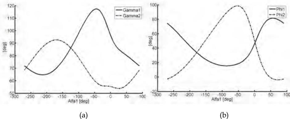
Fig. 6. Characterization angles of the right leg mechanism as function of angle  $\alpha_1$ : (a) angles  $\gamma_1$  and  $\gamma_2$ ; (b) angles  $\varphi_1$  and  $\varphi_2$
