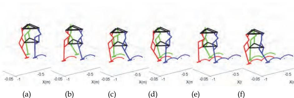
Fig. 14. Walking snapshots of the tripod walking robot as function of the input for leg motion: (a)  $\alpha_1=270$  degs; (b)  $\alpha_1=90$  degs; (c)  $\alpha_1=180$  degs; (d)  $\alpha_1=270$  degs; (e)  $\alpha_1=90$  degs; (f)  $\alpha_1=180$  degs
