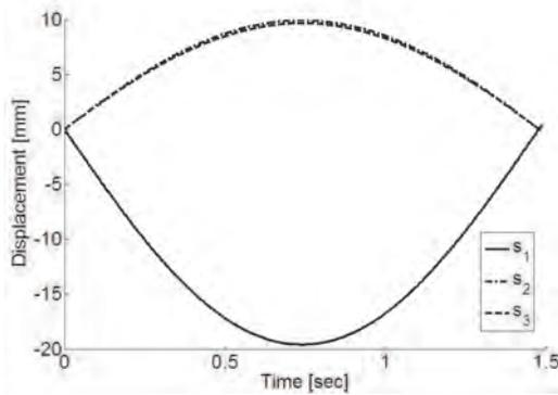
Fig. 34. Computed leg displacements of the waist module
