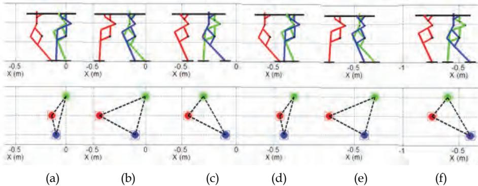
Fig. 15. Walking sequences and trajectories of the feet in sagittal plane and position of the three feet in horizontal plane: (a)  $\alpha_1=270$  degs; (b)  $\alpha_1=90$  degs; (c)  $\alpha_1=180$  degs; (d)  $\alpha_1=270$  degs; (e)  $\alpha_1=90$  degs; (f)  $\alpha_1=180$  degs
