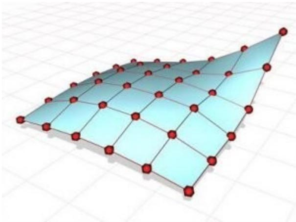
Of course there are situations where an approximate coding the 3D model is not enough and requires accurate encoding of the geometry of the surface. For example, during the construction of the body of an aircraft, especially a round hull, a discrete polygonal mesh will not work. Although the model may seem good for small resolutions, the flat surfaces and sharp angles become apparent closely.
