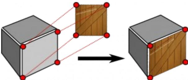
In the texture mapping, each point on the surface of the 3D model (or polygonal mesh) is mapped to a 2-dimensional image. The coordinates of the 2D image have attributes such as color and texture. When rendering of the 3D model, a coordinate is assigned to each surface point in the 2-dimensional image. The vertices of the mesh are mapped first. The coordinates of the other points are then allocated by interpolation between the coordinates of the vertices.
