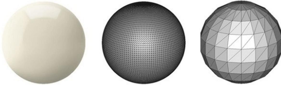
The approximate sizes or tiled are best used in situations where you do not need ultra-fine resolutions of the 3D model. A good example is 3D printing. 3D printers can not print beyond a certain resolution and, therefore, this type of 3D printing file format is ideal. In fact, 3D printing file format most popular, STL, actually belongs to this class of file formats.
