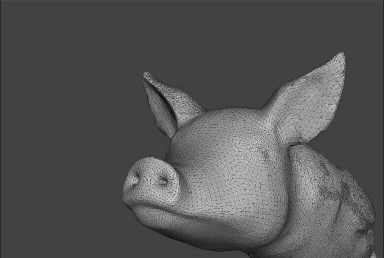
In this encoding, the surface of a 3D model is first covered with a tiny imaginary polygon mesh. Triangles are the most commonly used form. The tops of the collection of triangles and the normal vector coming out of the triangles are stored in the file. This represents the surface geometry of the target model.
