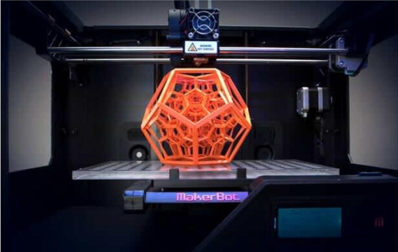
In 3D printing, high precision is not necessary because the current printers can not print beyond a certain resolution. Therefore, using the approximate file encoding formats of the surface geometry are ideal for the job. STL is one such file format and is the 3D printing format most widespread to date.
