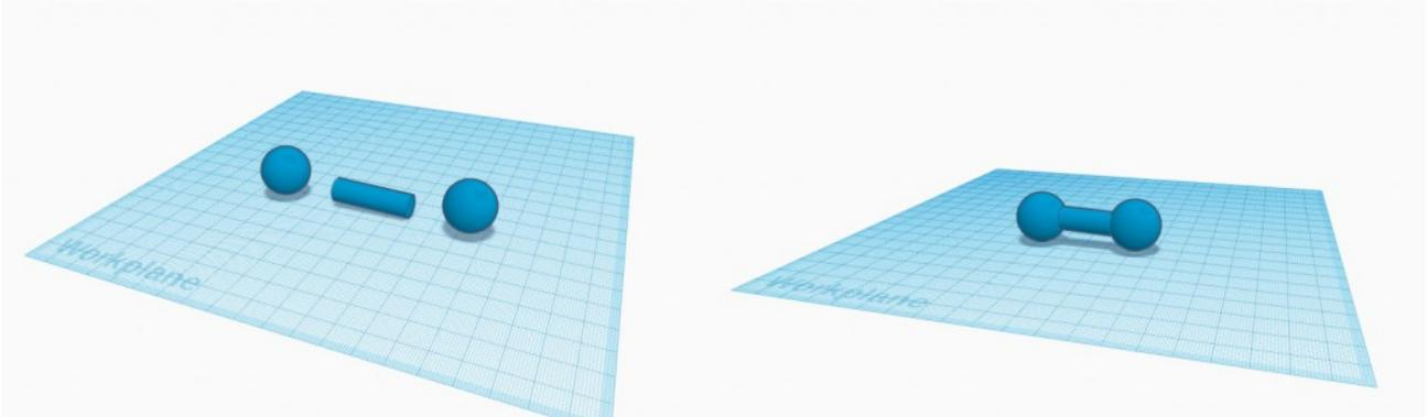
The solid constructive geometry is ideal for 3D models design and is very user friendly. Another great benefit is that each individual editing step (addition, subtraction, primitive forms of transformation) is stored in this 3D file format. Therefore, you can undo and redo any stage at any time.
