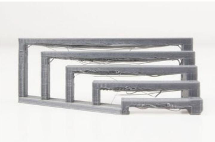
Poor, droopy bridges can also be corrected by adjusting flow rate in Cura. If filament is being extruded unevenly or at an excessive rate, material flowing from the nozzle will fall into a miserable mess.
