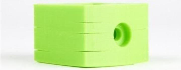
Layer delamination is a pesky 3D printing issue, but proper calibration of flow rate in Cura can be an easy fix.
