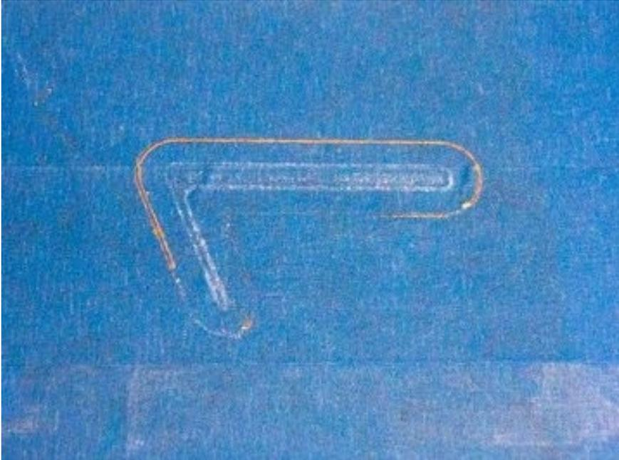
Ensuring your first layer sticks to the print bed effectively is paramount to good print quality. Poor bed adhesion will cause a print to fail almost every time. As such, you should alter your initial layer settings to ensure the print won't delaminate during the print, which wastes significant amounts of time and filament.
