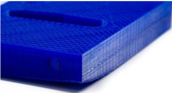
Prints popping off the plate is annoying; warping, equally so. To [improve print bed adhesion](#), you can try increasing flow rate in 5% increments. By increasing the amount of plastic extruded, the first layer should have a greater surface area with which to adhere to the print surface.
