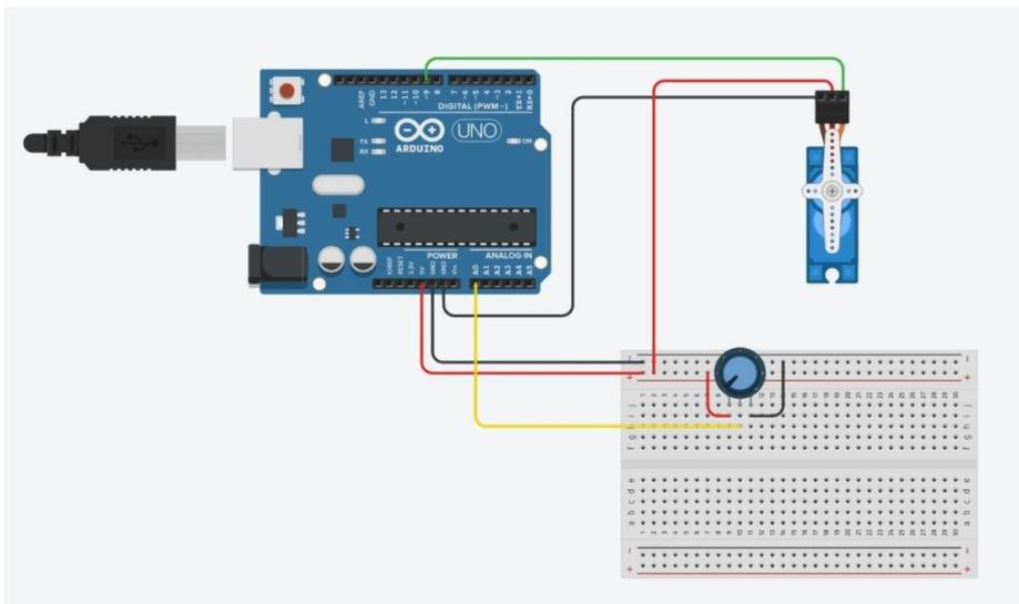
*Since the potentiometer is an analog component, we need to connect it to an analog input of our Arduino. The analog pins on the arduino are marked as A0, A1 etc. I have connected the potentiometer to the A0 pin.*
