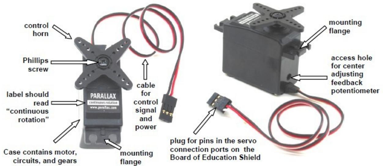
It is worth noting that continuous servos **do not offer exact position control** of the shaft.
