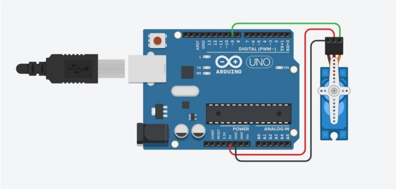
**NOTE:** To minimize the risk of drawing too much current and damaging your USB port, do not put heavy loads on the motor. If you need the motor to control the position of something, please connect an external 5V (or a supply that can provide the operating voltage of the motor) supply as shown in the diagram below.
