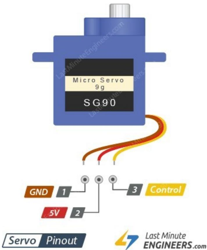
The brown and red pins are the power pins, and the yellow pin is the signal input pin.
