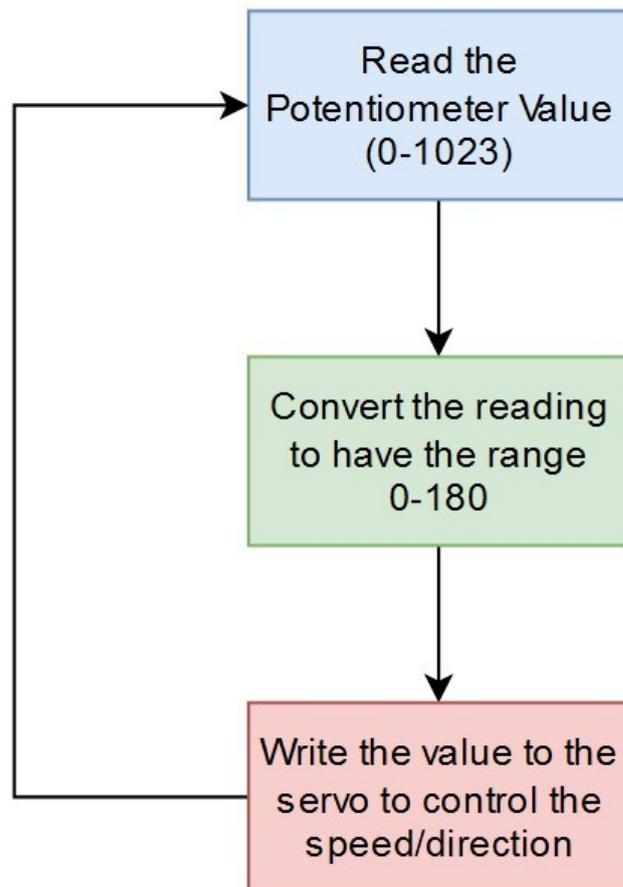
The `val = analogRead(potentiometerPin);` line reads the potentiometer reading, and assigns it to the variable ***val***.
