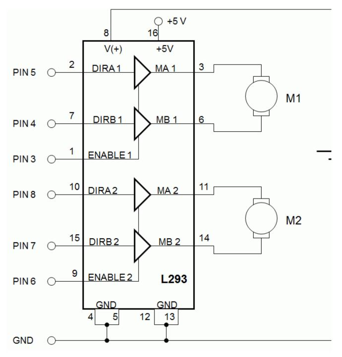
Assume you have only one motor connected with the enable tied to Arduino Pin 3, and the two direction controls tied to Arduino Pins 4 and 5.
