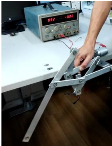
Figure 6: Aluminium Klann Linkages
