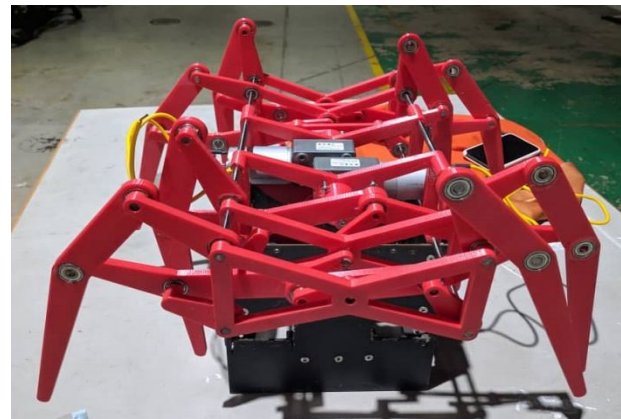
Figure 8: Two motors are placed at the centre of the robot. Each motor drives four Klann linkages.
