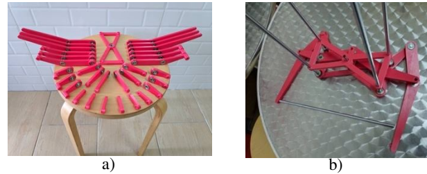
Figure 7: a) 3D printed parts of the robot made using PETG material. b) Parts were assembled with rods.
